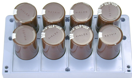
Capacitor Bank for DC Link (See Chapter 6 for servicing)
